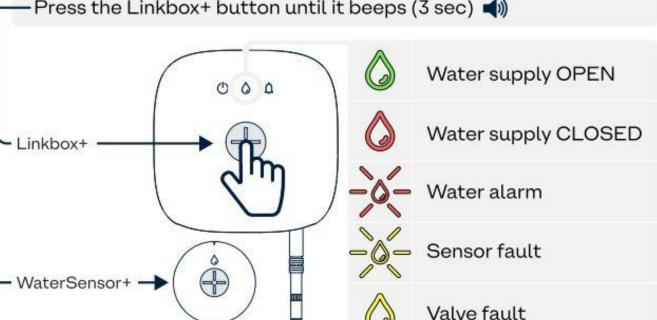
Required to test the system twice a year. Dampen the water sensor and validate that the water supply is shut off. Disable the alarm and repeat on all water sensors.
